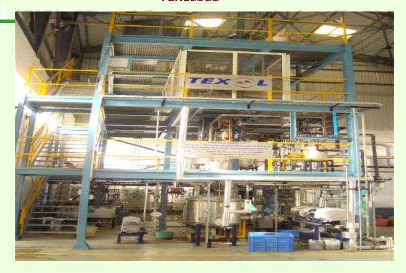
Multi feed Lignocellulosic Biomass to ethanol pilot plant in collaboration with NREL USA(5-8 Kg/hr multi feed capability)
