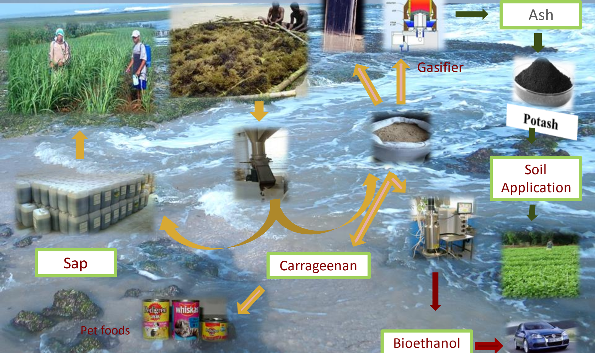
Integrated process for utilization of Kappahycus for biopotash, bioethanol and energy
